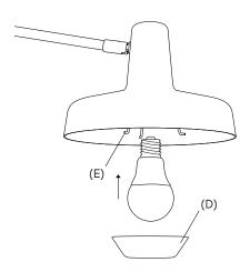
5. To insert the light bulb, release the undershade (D) by pressing three undershade brackets (E) inwards.
