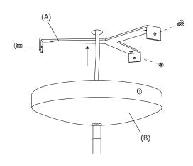
4. Attach the lamp body back to the ceiling mounting.
