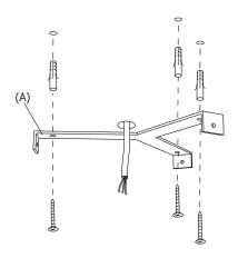
Mount the ceiling mounting to the ceiling with three appropriate screws and plugs. Always use correct screws and plugs for the mounting surface.
