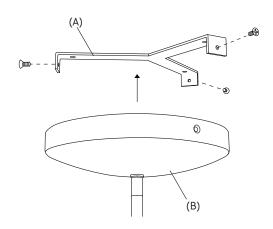
1. Remove the ceiling mounting (A) by unscrewing three screws from the lamp body (B).
