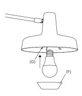
To insert the light bulb, release the undershade (F) by pressing three undershade brackets (G) inwards.
