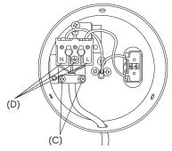
Unscrew the two screws (C) from the back of the lamp housing. Press N, ⊕, L tabs (D) on terminal strip to pull the cord out.
