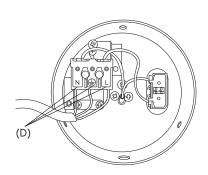
4. Connect the electrical cord with the terminal strip (D).
