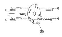
3. Position the wall mounting making sure the metal handle (E) is covering the hole on the lamp body. Mount it with four appropriate screws and plugs. Always use correct screws and plugs for the mounting surface.
